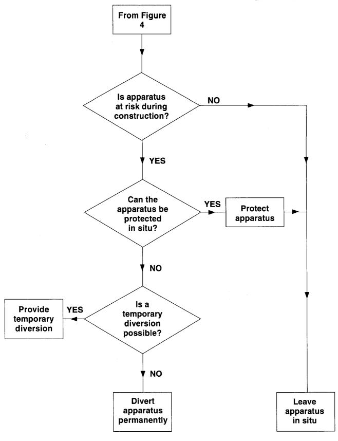
FIGURE 3 APPARATUS AT RISK DURING CONSTRUCTION
